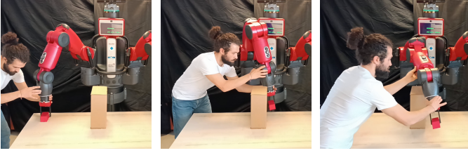
Fig. 5. Demonstrations of the obstacle avoidance skill are being performed by an expert. Kinesthetic teaching is used to generate sensorimotor demonstrations. Later, this data is used to train CNEP and CNMP models.
